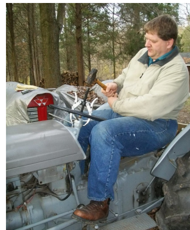
While using legs to apply upward pressure on the steering wheel, swift strikes with a hammer are applied to shock the steering wheel loose.
