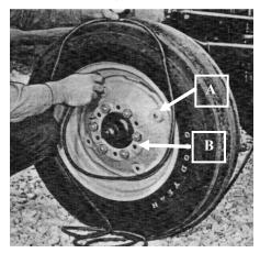
This photo of a Ferguson tractor shows the correct rim configuration. Note the four round holes (A) for mounting wheel weights on the inside of the rim. The area around the hole is raised to the outside of the rim. (B) shows one of the 12 mounting holes that are finished on both sides so that the rims can be reversed and still have a flat surface against the hub.
