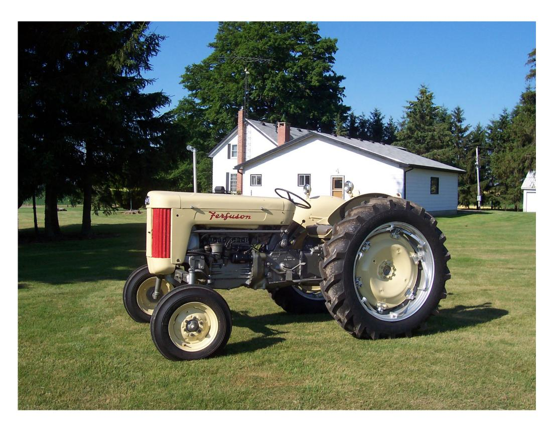
**Donald Martin of Burford, Ontario, Canada's 1956 Ferguson 40, High Arch,** with spin out rims, power steering and vertical exhaust. It had been on a small farm with a manure loader mounted on it since
