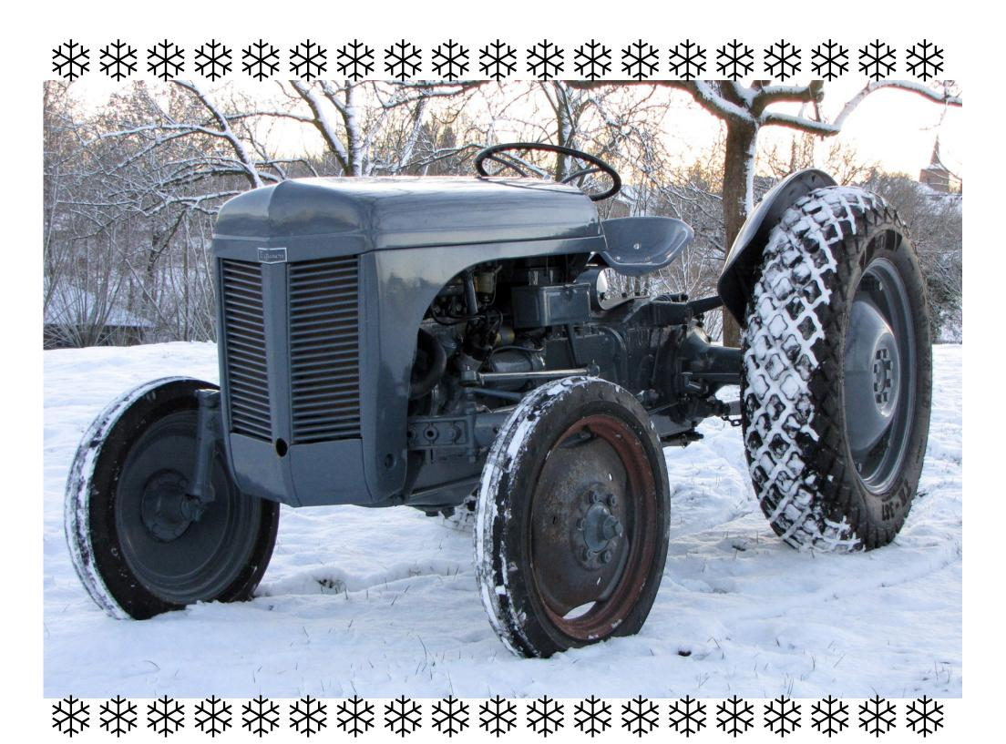
**Thomas van der Luit of Epen, Limburg, Netherland's, TE 20** shown above was restored in 2008. It's fully original, only a new paint job and overhaul of the engine was needed after 60 years of service, Note the later type front wheel, they replaced temporary due to a flat tire!
